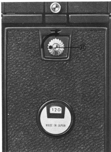
Twist the back cover catch button (31) until the red mark on the button faces upward. Then, by pressing the button in the direction indicated on the back cover, the back cover will open. The figure in the exposure counter automatically returns to "0" when the back cover opens.
