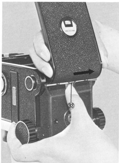
The back cover of this camera can be exchanged with the exclusive back cover for single exposure attachment. Release the back cover catch button and open the back cover halfway. In this condition, slide the back cover in the arrow direction (as shown in the picture) while depressing the back cover hinge release (33).
