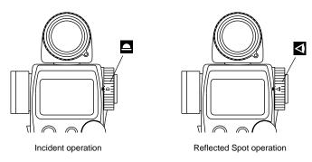
When incident operation is selected, the mark will blink for three seconds and when Reflected Spot operation is selected the mark will blink for three seconds on the LCD.
