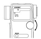
Press the Measuring button (4) to trigger the flash.
