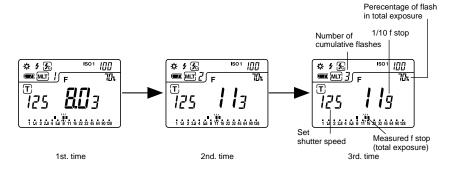
5. To clear the cumulative value, press M. CLEAR button ② or switch to another mode by turning the Jog wheel while pressing the mode set button.
