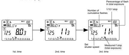
3. The ready to measure mode will be displayed for approximately 90 seconds. If the 90 second period is exceeded and the blinking mark stops, press the Measuring button (3) again. The measured value (f stop) of the previous time reverts to 0 and the meter is in ready to measure mode.
