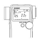
4. Turn the main lighting off. Now, point the Lumisphere toward the secondary light source. While the Measuring button (1) is depressed and held down, the indicated difference between the main and auxiliary light sources is displayed in EV values. At the same time, the standard value and a new measured value are displayed on the analog scale.
