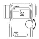
Press the Measuring button (4) to make a measurement.
