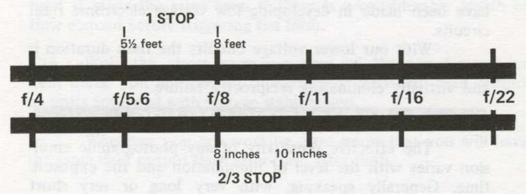
This same system can be used to determine exposure increase needed for bellows extension. From the lower side of the scale you can see that if you are using an eight inch lens and the bellows are extended to ten inches, you would need to increase exposure by 2/3 of a stop.
