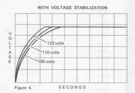
Voltage stabilization is vitally important to light output consistency from an electronic flash unit and is best demonstrated by the two graphs here.
