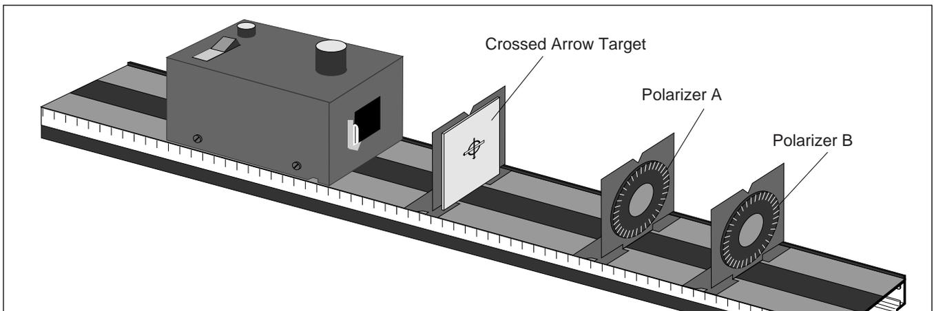
Figure 10.2 Equipment Setup
