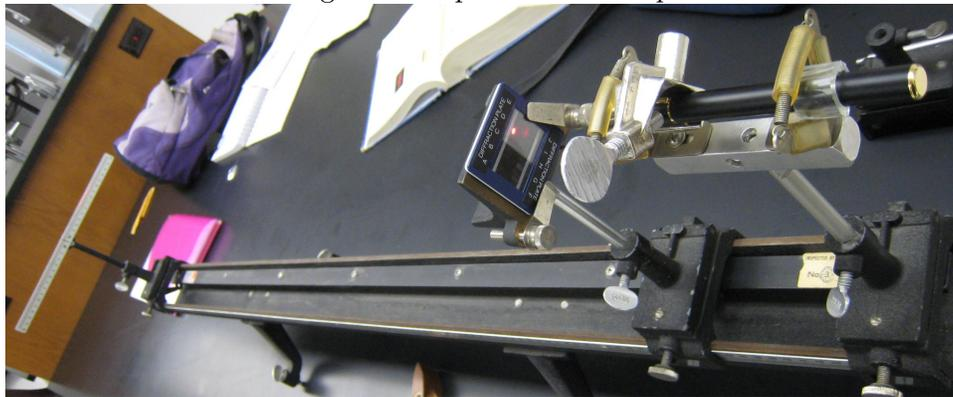
2. Measure the distance between the first two dark fringes then follow the calculation above to calculate the wavelength. Do this for slits A, B and C. Find the average wavelength from these three cases.
