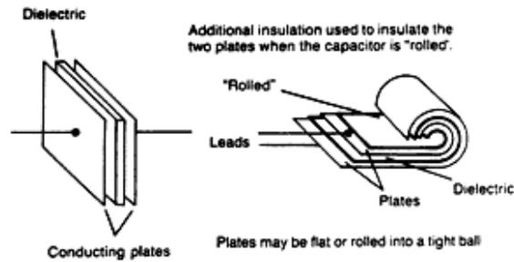
Figure 1: Capacitor Construction
